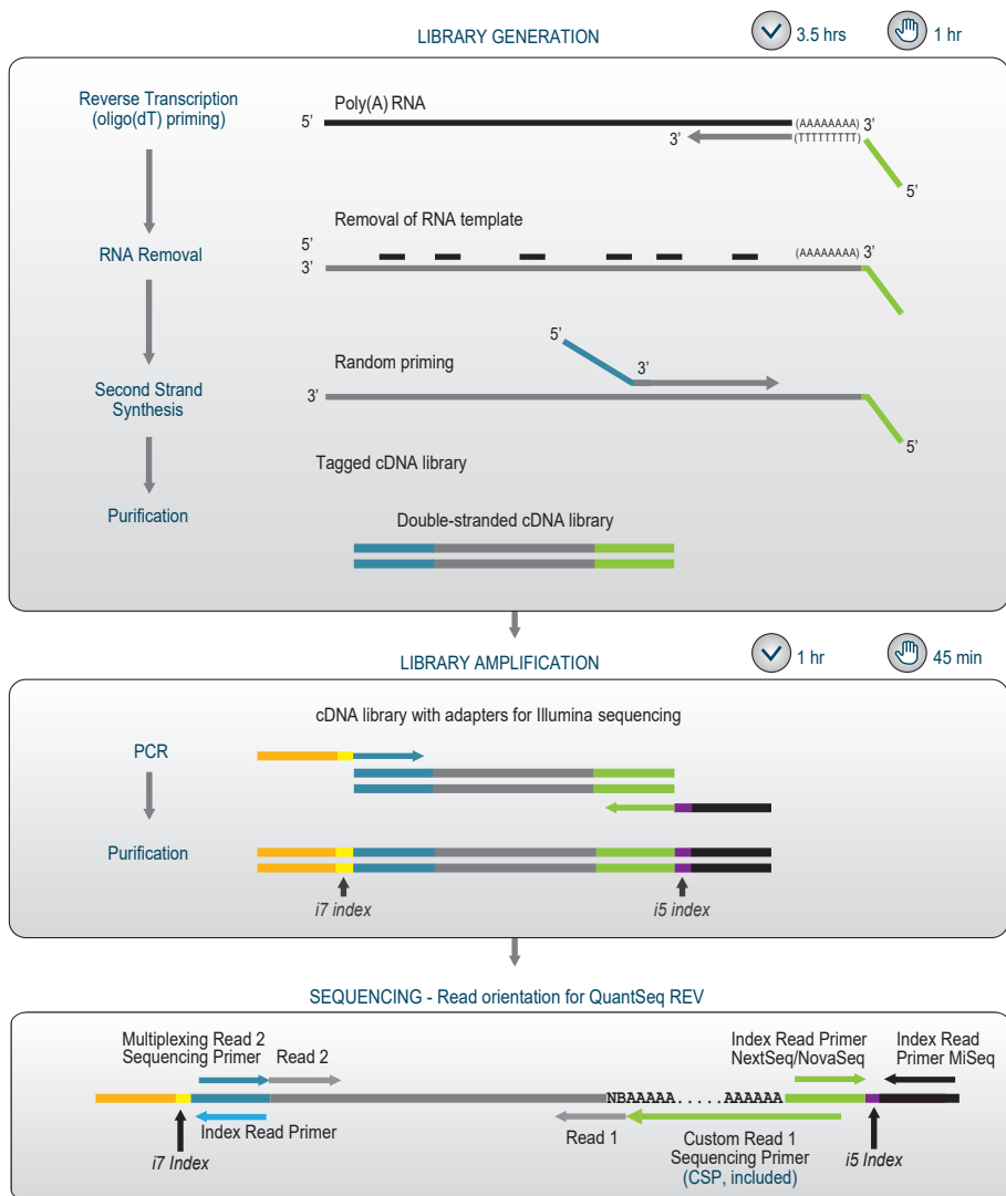
Figure 1. Schematic overview of the QuantSeq REV V2 library preparation workflow (Cat. No. 225). Sequencing read orientation for QuantSeq REV is depicted, with Read 1 (green) and Read 2 (blue). Read 1 reflects the cDNA sequence. QuantSeq REV is suitable for paired-end sequencing, and Read 2 reflects the mRNA sequence. A Custom Sequencing Primer (CSP Version 5, included in the kit) is required for Read 1.
