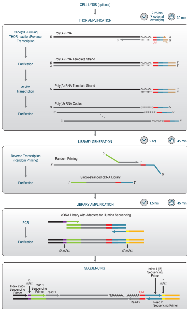
Figure 1. Schematic overview of the LUTHOR HD 3' mRNA-Seq library preparation workflow (Cat. No. 204). Partial P7 sequences are shown in blue, partial P5 sequences in green, Unique Molecular Identifier (UMI) in red, and T7 promoter sequences in light brown. Sequencing read orientation for LUTHOR HD is depicted, where Read 1 reflects the mRNA sequence, while a 12 nt long Read 2 is required for UMI read-out.
